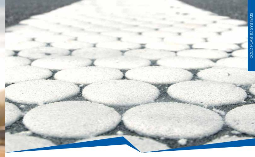
Cold plastic marking materials are based on acrylate binder and reactive monomers, where curing takes part upon the addition of a catalyst. Known for the highest endurance amongst all marking materials, they are offering supreme durability. As solvent- and VOC-free option, they provide one of the most environmentally friendly road marking solutions according to life-cycle assessments.
