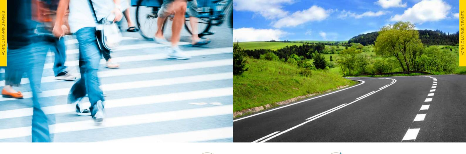
Acrylic marking paints provide a solution enabling easy application. These paints are durable and fast-drying and are used for road markings in thicknesses of up to 600 microns by conventional marking machines.
